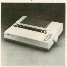
ing the high quality of its printed output. **Antic** tested the speed of this printer at 105 characters per second in draft mode and 20 cps in near letter quality mode. The FX-85 also seems much quieter than many of its competitors.
